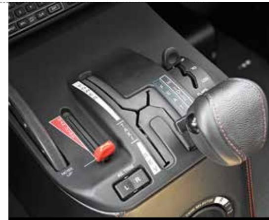
THE TBM 900'S NEW POWER QUADRANT MECHANICALLY COMBINES POWER, CONDITION AND PROP LEVERS, CREATING AN INGENIOUS SINGLE-LEVER SOLUTION.
