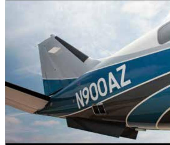
A NEWLY DESIGNED VENTRAL FIN GIVES THE TBM GREATLY ENHANCED SLOW SPEED AND HIGH-POWER CONTROLLABILITY, ALLOWING THE AIRPLANE TO USE FAR GREATER TAKEOFF POWER.
