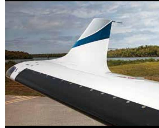
THE WINGLETS, NEW ON THE 900, IMPROVE THE TBM'S PERFORMANCE, CUTTING DRAG AND IMPROVING THE FEEL AND ACCURACY OF THE AILERONS.
