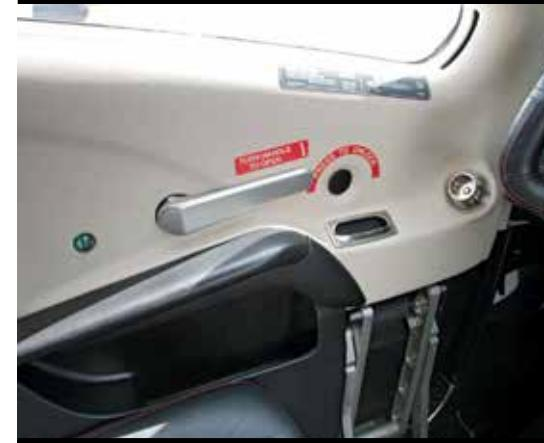
STANDARD ON THE 900 IS A PILOT'S DOOR, WHICH WAS FORMERLY AN OPTION. THE DOOR LOOKS THE SAME BUT HAS BEEN STRUCTURALLY REDESIGNED TO BE MORE DURABLE AND EASIER TO OPERATE.
