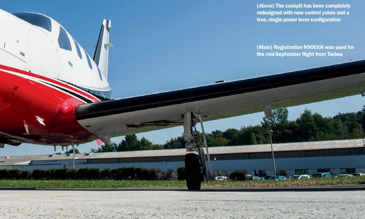
» in-house expertise) now accounts for nearly 25% of the aircraft's structure. Possibly the most obvious external difference is the new, highly swept, carbonfibre, five-bladed Hartzell propeller, which still features full reverse capability. The wings now have 0.6m (2ft) carbonfibre composite winglet extensions (to TBM's own design).
