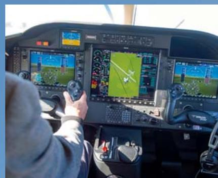
(Above) The cockpit has been completely redesigned with new control yokes and a true, single power lever configuration
