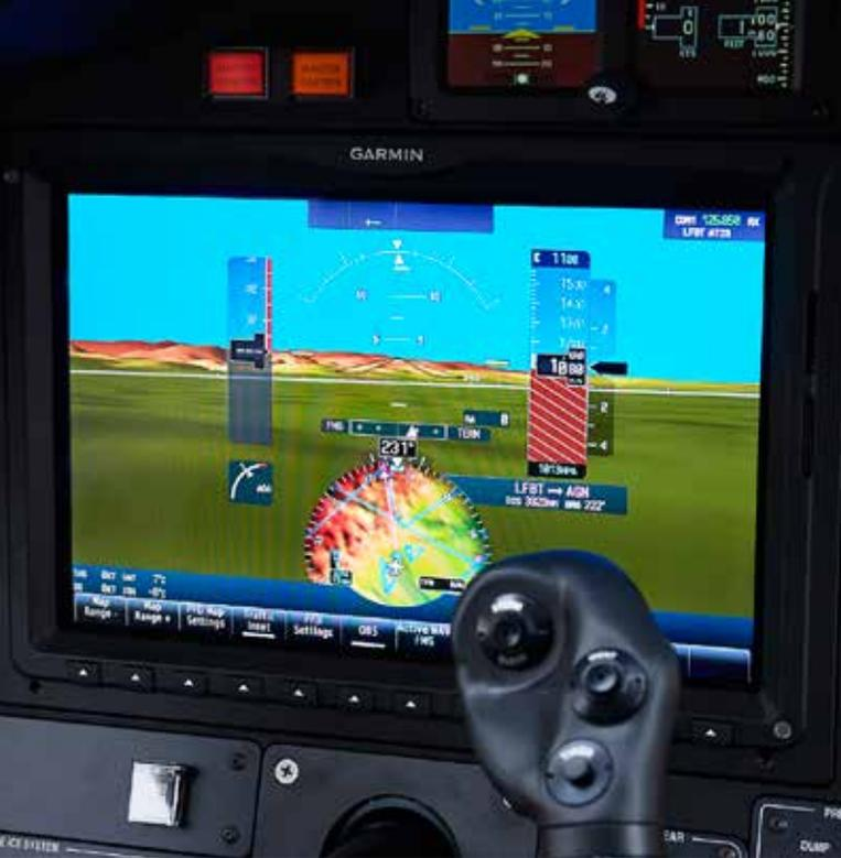
**THE 930'S G3000** primary flight display (above, left) has a feature that lets you move the screen's inset map from the screen's lower left into the compass rose. Also standard is Mid-Continent's new MD302 standby instrument package (above, right), which has a self-contained battery and measures 2.4 inches by 5.5 inches.
