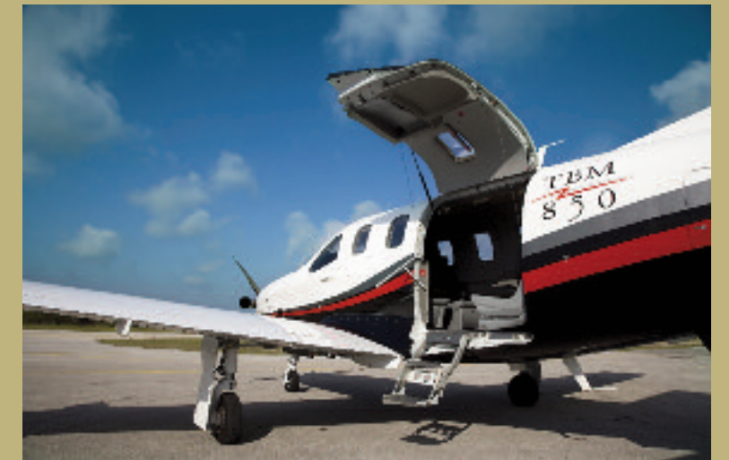
The larger, electrically actuated door carries over from the TBM 700C models.
