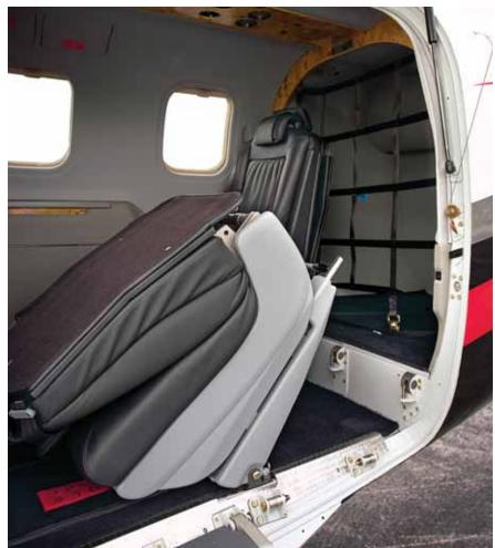
The club-style passenger area (top) has been changed slightly to give more shoulder room, and a single storage cabinet is now standard. A second cabinet with a CD player is a \$5,600 option. Aft seats (above) fold forward for loading the aft baggage compartment.
