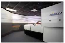
training devices, is built from a real airplane cockpit. The cockpit with an instructor cab built onto the back of it sits in a large room. Projectors driven by a bank of computers project environmental images on the walls around the cockpit. The cockpit doesn't move, but you wouldn't know it when you're inside. The moving images convince your brain that you are in fact moving. It's an amazing technolo-
