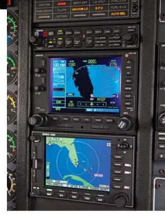
Most TBM 700s and 850s leave the factory with Honeywell Bendix/King's IHAS (integrated hazard avoidance system) 8000 avionics package. This \$61,300 option includes TAS (traffic alert system), TAWS (terrain awareness warning system), and Stormscope information, presented on the centrally mounted Bendix/King KMD 850 multifunction display. Dual Garmin 530 GPS/nav/coms and a GTX 330 transponder with TIS (traffic information system) are standard.
