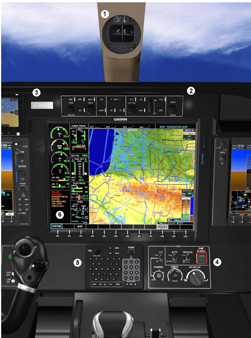
Figure 7.3.4 (2/2) - Central instrument panel (Typical arrangement)
