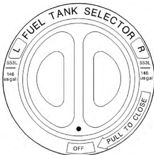
Figure 7.7.2 - Manual selector of fuel tanks
