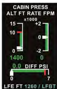
Figure 7.9.1 - Cabin altitude monitoring
