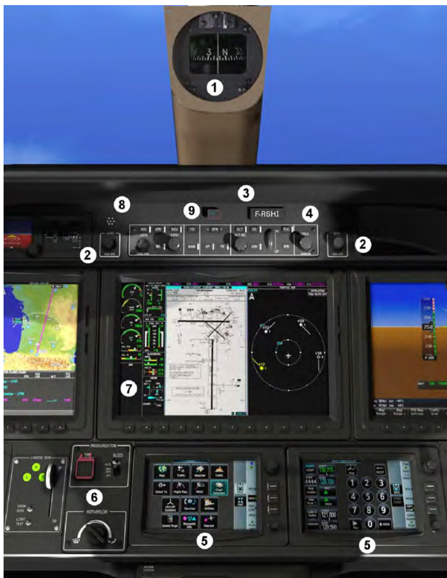
Figure 7.3.4 (2/2) - Central instrument panel (Typical arrangement)
