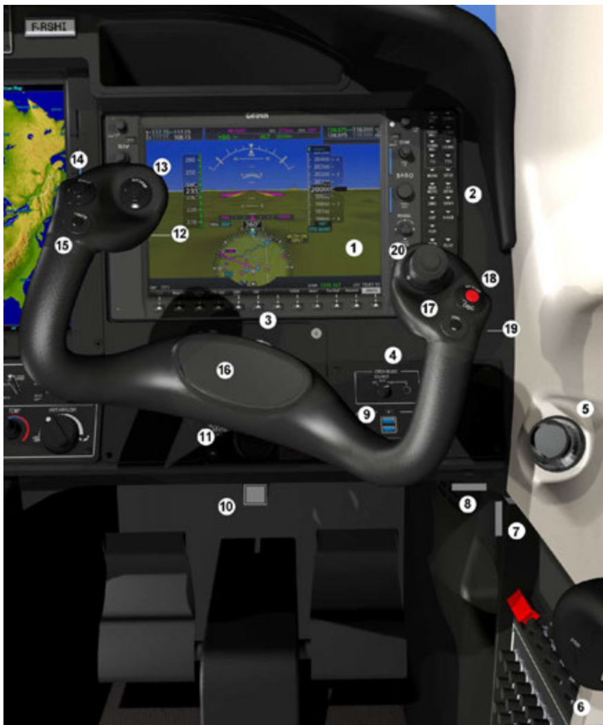
Figure 7.3.5 (2/2) - Right instrument panel (Typical arrangement)
