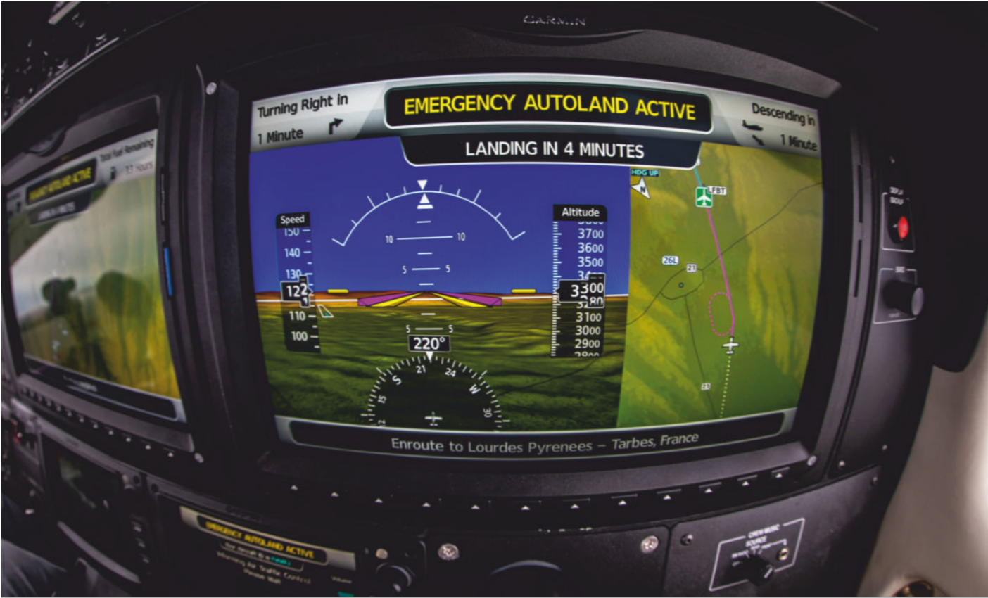
ABOVE: A big part of autoland, Daher and Garmin knew, was making sure that passengers were kept calm and in the loop. Part of that is communicating clearly and calmly from the outset of HomeSafe activation. BELOW: Hands in the lap, Daher's demonstration pilot lets HomeSafe do all the work.
