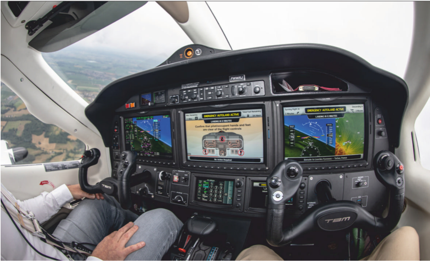
ABOVE: A big part of autoland, Daher and Garmin knew, was making sure that passengers were kept calm and in the loop. Part of that is communicating clearly and calmly from the outset of HomeSafe activation. BELOW: Hands in the lap, Daher's demonstration pilot lets HomeSafe do all the work.
