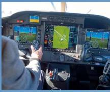
(Above) The cockpit has been completely redesigned with new control yokes and a true, single power lever configuration
