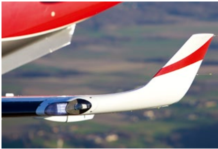
Winglets add dihedral and allow full power to be used on take-off, unlike the TBM 850 which was physically limited to 700shp
