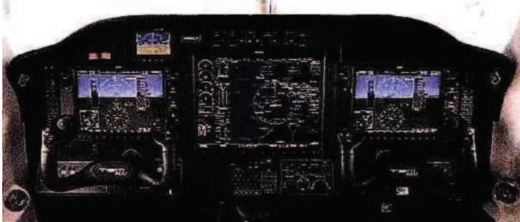
Like the TBM 850, the TBM 900 includes the popular G1000 avionics suite from Garmin. It will, however, feature several human-machine interface improvements from the 850.
