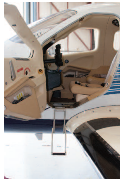
The TBM 850 features pilot doors and a separate passenger/cargo door that's electrically operated and swings open upward with fold-out airstairs that swing down.
