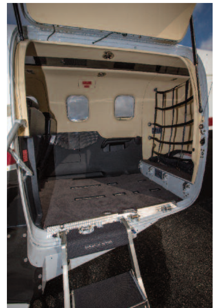
The TBM 850 features pilot doors and a separate passenger/cargo door that's electrically operated and swings open upward with fold-out airstairs that swing down.
