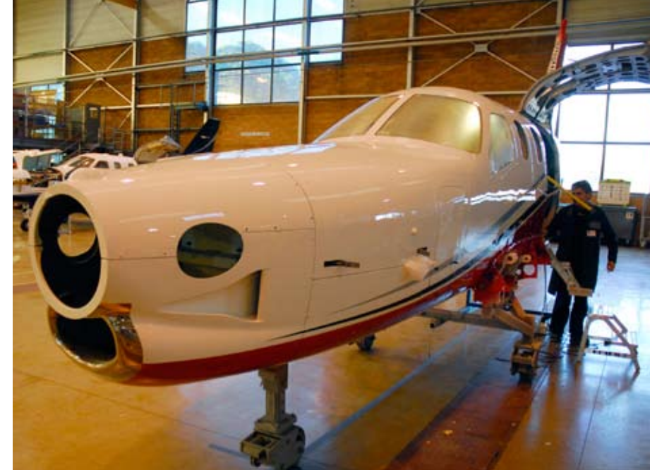
Left: fitting out a freshly-painted standard-build fuselage in the main assembly hall at Tarbes
