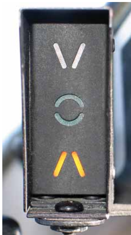
Angle of attack indexer shows “nose up” chevron illuminated, indicating that airspeed is fast, and the pilot should raise the nose.
