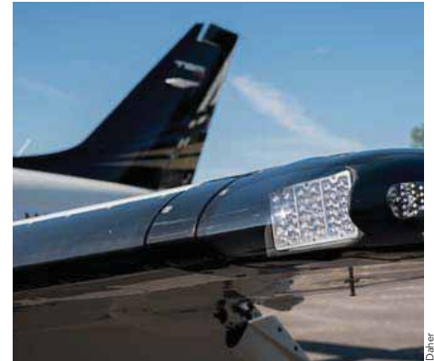
Booted leading edges offer anti-icing aid
