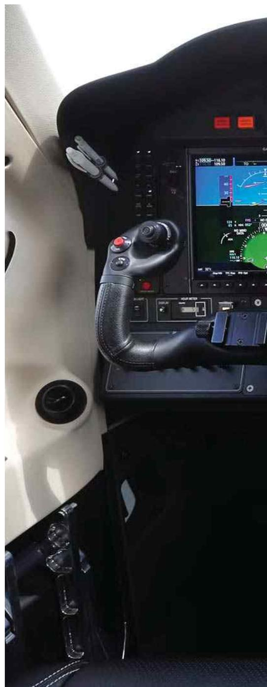
**CLOCKWISE FROM TOP LEFT:** The G1000 NXi-equipped TBM 910 retains Garmin’s legacy keypad data-entry interface; new touches from the TBM 930 include a clean look for the subpanel, USB charging ports, and a single-lever power control with twin functions. The left side of the H-shaped control gate provides thrust, beta, and reverse thrust. Slide the lever to the right side and it acts as a condition lever. The NXi’s screens initialize faster and have higher resolutions than their predecessors.
