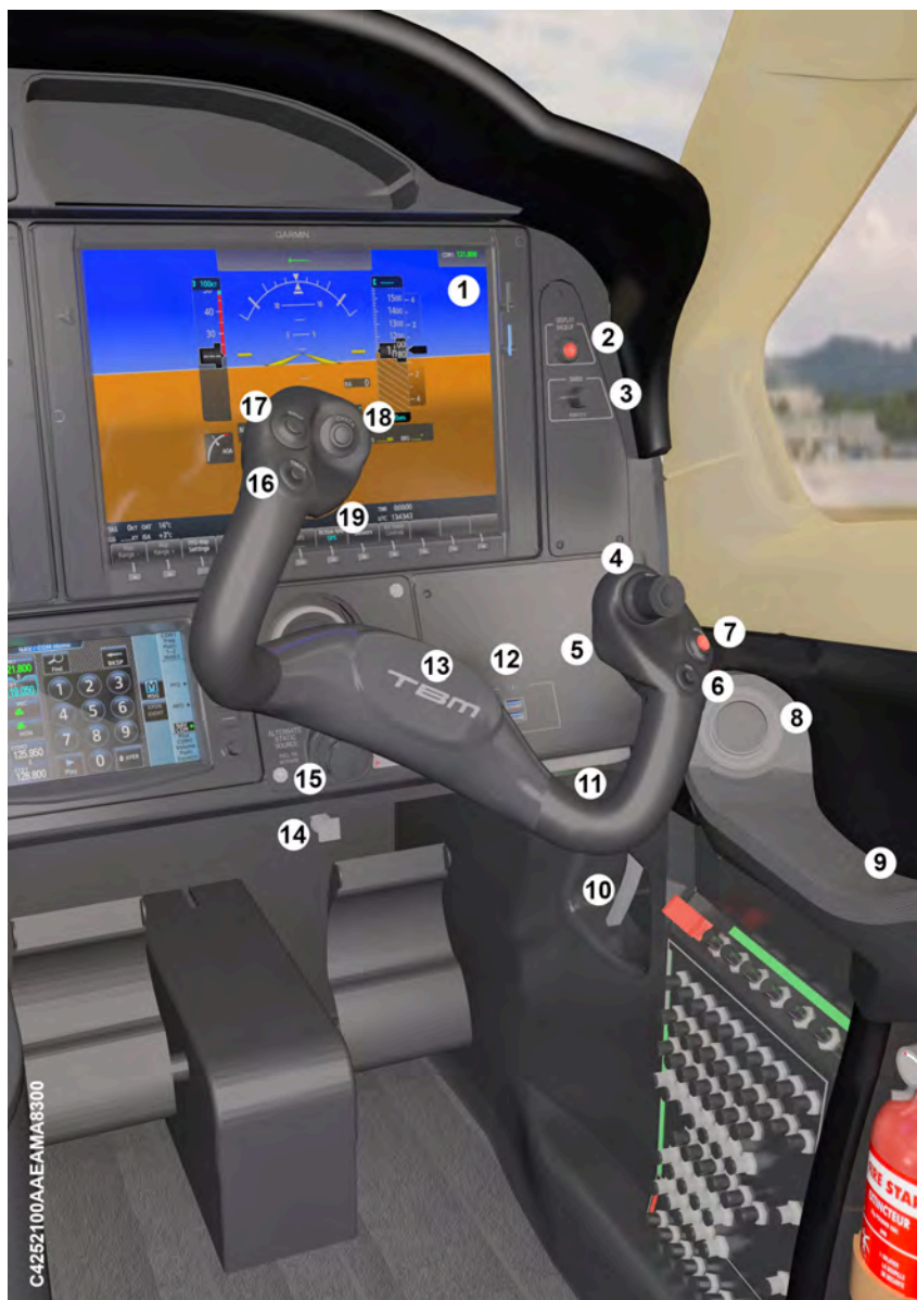
Figure 7.3.8 - Right Instrument Panel (Typical arrangement)
