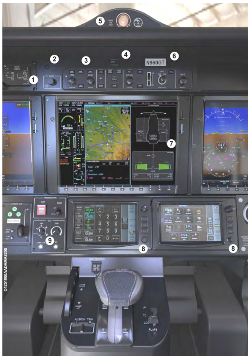
Figure 7.3.4 - Central Instrument Panel (Typical arrangement)
