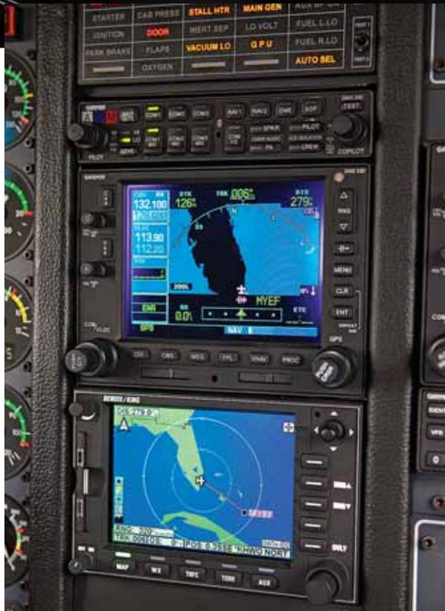
Most TBM 700s and 850s leave the factory with Honeywell Bendix/King's IHAS (integrated hazard avoidance system) 8000 avionics package. This \$61,300 option includes TAS (traffic alert system), TAWS (terrain awareness warning system), and Stormscope information, presented on the centrally mounted Bendix/King KMD 850 multifunction display. Dual Garmin 530 GPS/nav/coms and a GTX 330 transponder with TIS (traffic information system) are standard.
