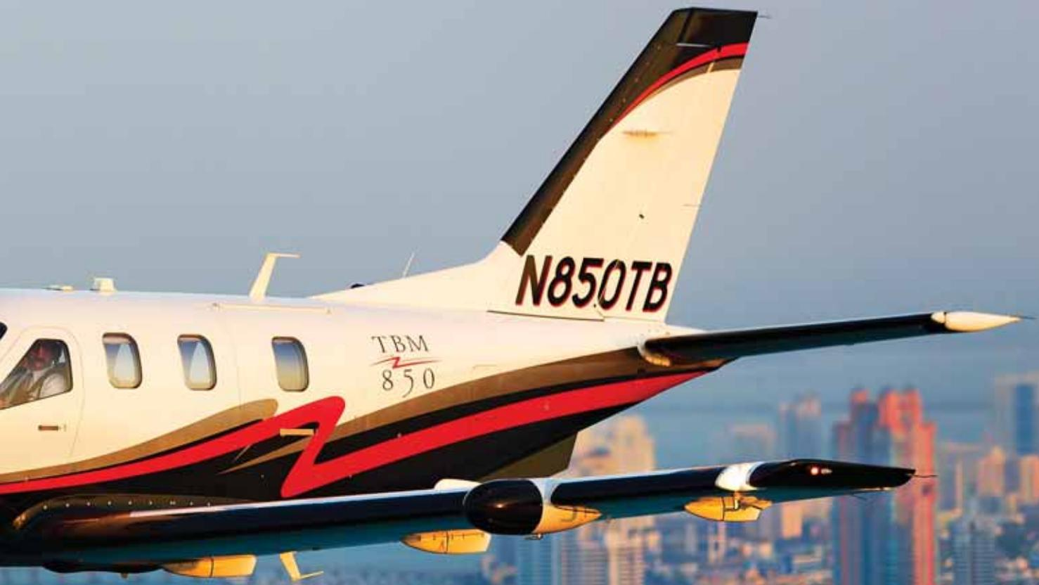
improvements over the TBM 700's climb performance. Under hot and high (international standard atmosphere plus 20 degrees) conditions the TBM 850 climbs to FL310 in half the time it takes the TBM 700. That's important because turbine aircraft burn much less fuel at altitude, so the faster you can climb to higher altitudes the lower your total fuel consumption.
